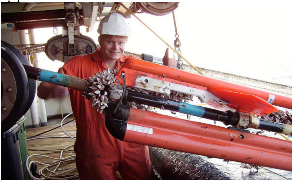
Fig 12. Barnacle growth on streamer depth controller.
